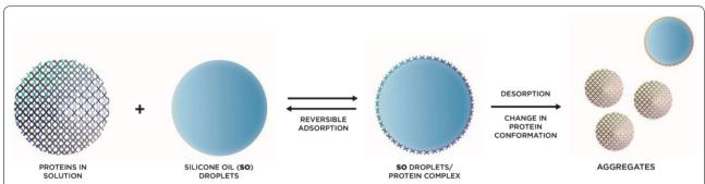
**Fig. 1** Schematic drawing illustrating possible interactions between silicone oil (SO) and proteins in solution. Proteins may undergo conformational change and film formation after interaction with the silicone oil surface. Fragmentation of SO-protein complexes results in smaller aggregates and agglomerates
